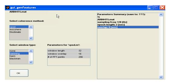
Figure 14. Features Module window for selecting coherence methods and setting parameters.
